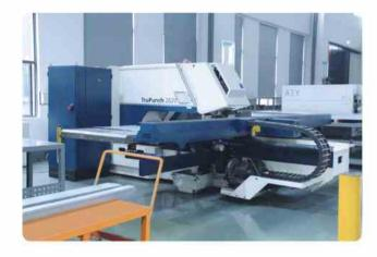
German Trumpf laser cutting and Trupunch ensures ±0.1mm accurancy for sheet-metal parts.
