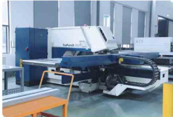
German Trumpf laser cutting and Trupunch ensures  $\pm 0.1\text{mm}$  accuracy for sheet-metal parts.
